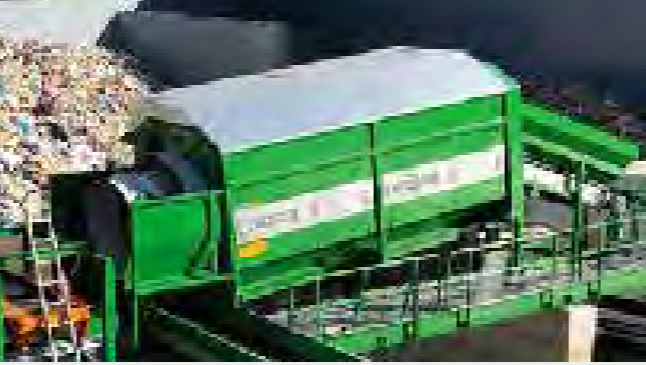
WEATHER OR DUST PROTECTION ROOF
